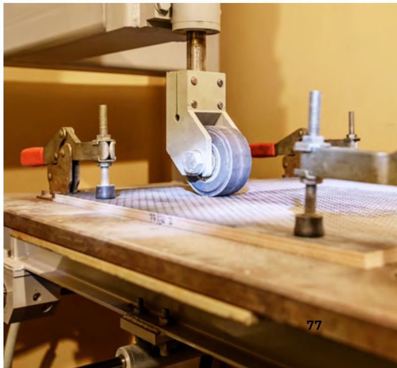
Figure 3.4. Determination of the effect of loaded heavy duty castors
